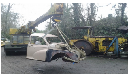
Cab lifted off by crane
