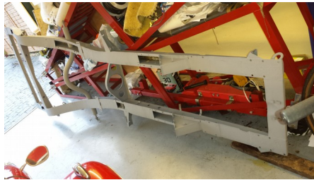
Sand blasted and in primer
